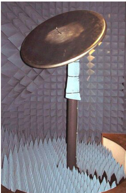
Figure 2-Ground plane used in SDARS type approval testing
