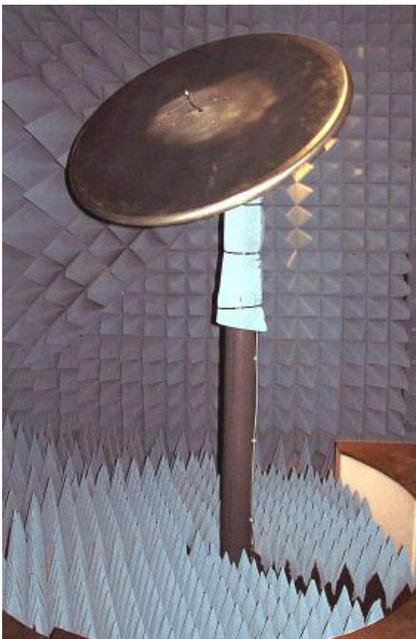
Figure 2-Ground plane used in SDARS type approval testing
